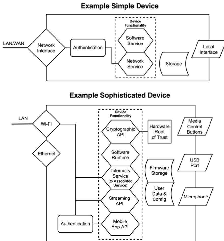
**Figure A.1: Examples of a general architecture of a device and of an architecture for a Smart Speaker**
