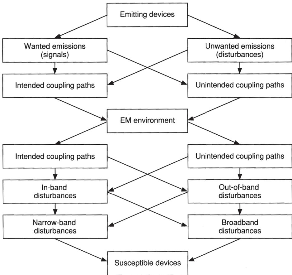
Figure 1.3 - EMI diagram: susceptible devices located in EM environment set up by emitting devices.
